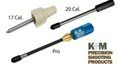
With the precision K & M uniformer you simultaneously "ream", "de-burr", and "chamfer" the inside of the flash hole. The unique feature of the K & M tool is that it provides uniformity with a "pre-set" depth stop surrounding the steel cutter; it does not require the cases to be trimmed to a uniform length. A "reversible" sliding "centering cone" is supplied to keep the case aligned and centered during the uniforming operation. These tools are designed with hand power in mind.
